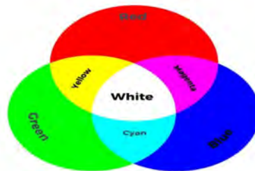
Figure 3. Concept of colour mixing individual red, green and blue LEDs [3]
