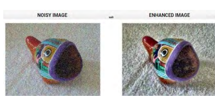
Figure 3: Original color image with salt and pepper noise (left), enhanced image (right)
